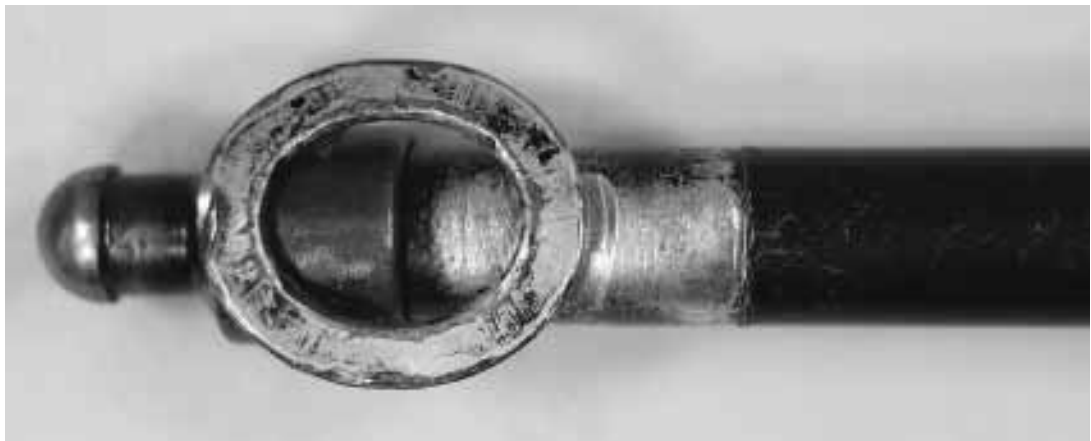
Figure 2. The deformed thrust washer and the deep rub marks on the push rod.
