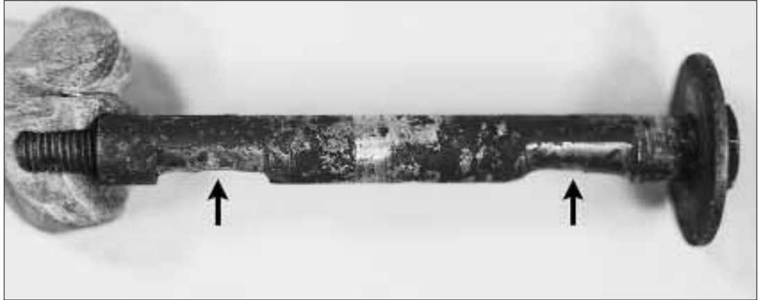
Figure 4. The worn pulley block securing bolt.
